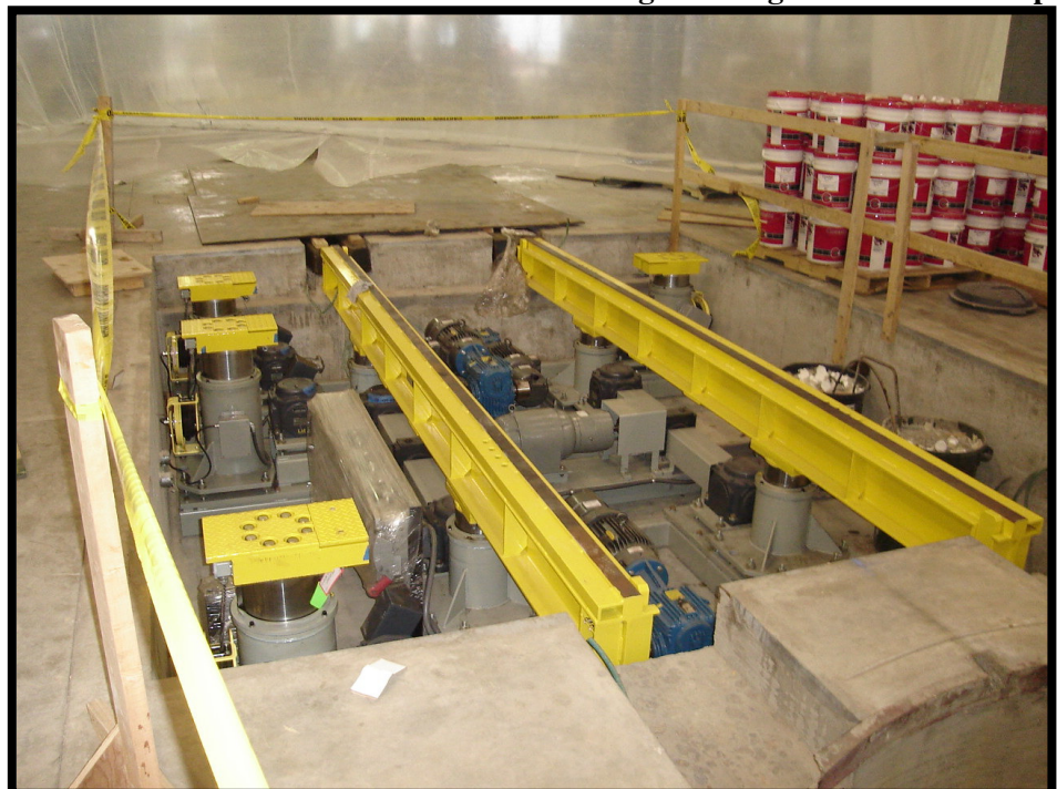
New Truck Hoists in Existing Running Maintenance Shop
